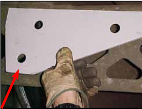
Locate Reinforcing Plate to the outside of the Sand Bracket - as shown.
